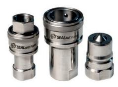
These couplings have automatic shut off valve at both ends; in socket & plug also. So on disconnection both socket & plug are sealed instantly. This type is widely used on Hydraulic lines carrying oils, water, chemicals & petroleum products. Material & seal are selected to suit the type of fluid.
