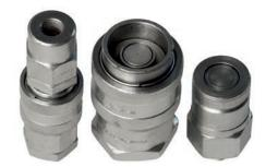
These couplings are designed for high pressure applications. As there is no air gap between plug & socket when connected, there is no chance of any air entering hydraulic lines, so air bleeding is unnecessary. Fluid leakage at the time of connection or disconnection is nil because it flows through the holes at the center of the valve body. Designed to provide one touch connection.
